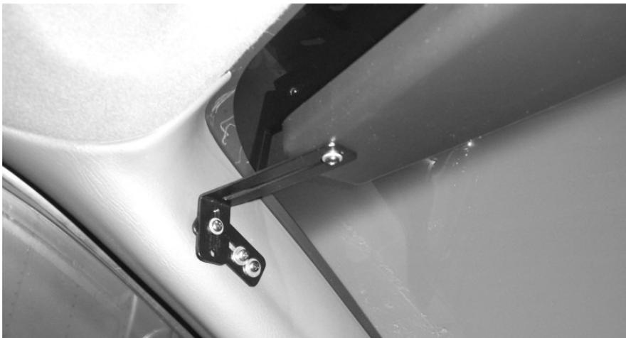
5. Adjust the mounting brackets so that they rest flat against the corner post on each side of the vehicle.
